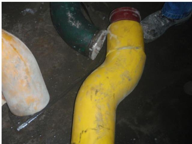
Distortions like the one shown in the following photo indicate that the CDD will be worn out soon. This is normal and shows no situation of danger. In this case the CDD is to be replaced soon. Therefore a new CDD is to be kept ready in order to keep interruptions as short as possible.
